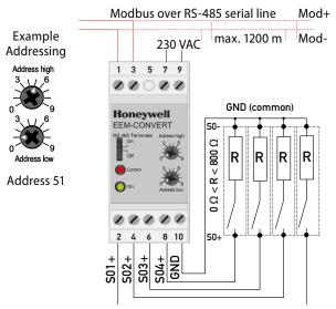
Note: If the S0-Modbus module is used in the Modbus as last device, then the sliding switch «RS-485 Terminate» need to be in the position «On».
